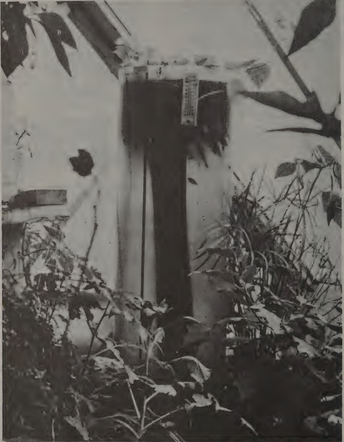
Inside the test model for the Cape Cod ark. Amid a diversity of tropical and food plants, a "solar tube" traps and stores solar energy while culturing algae and fish. Sunlight enters the building through one layer of Kalwall and three layers of the Suntek membrane developed by Day Charoudi and Sean Wellesley-Miller. The habitat remains tropical in mid-winter Massachusetts.
